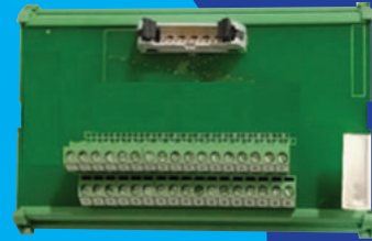
MAS-P-F25-M/MAS-P-F25-F FRC (PLC Side) to Screw Terminals (Field Side)
