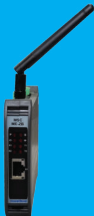
MSC-ME-ZB (Modbus-Zigbee to Modbus TCP/IP Data Concentrator/Gateway)
