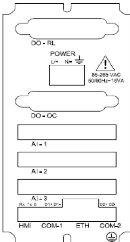
Figure 4 Rear Panel Diagram for AC Supply
