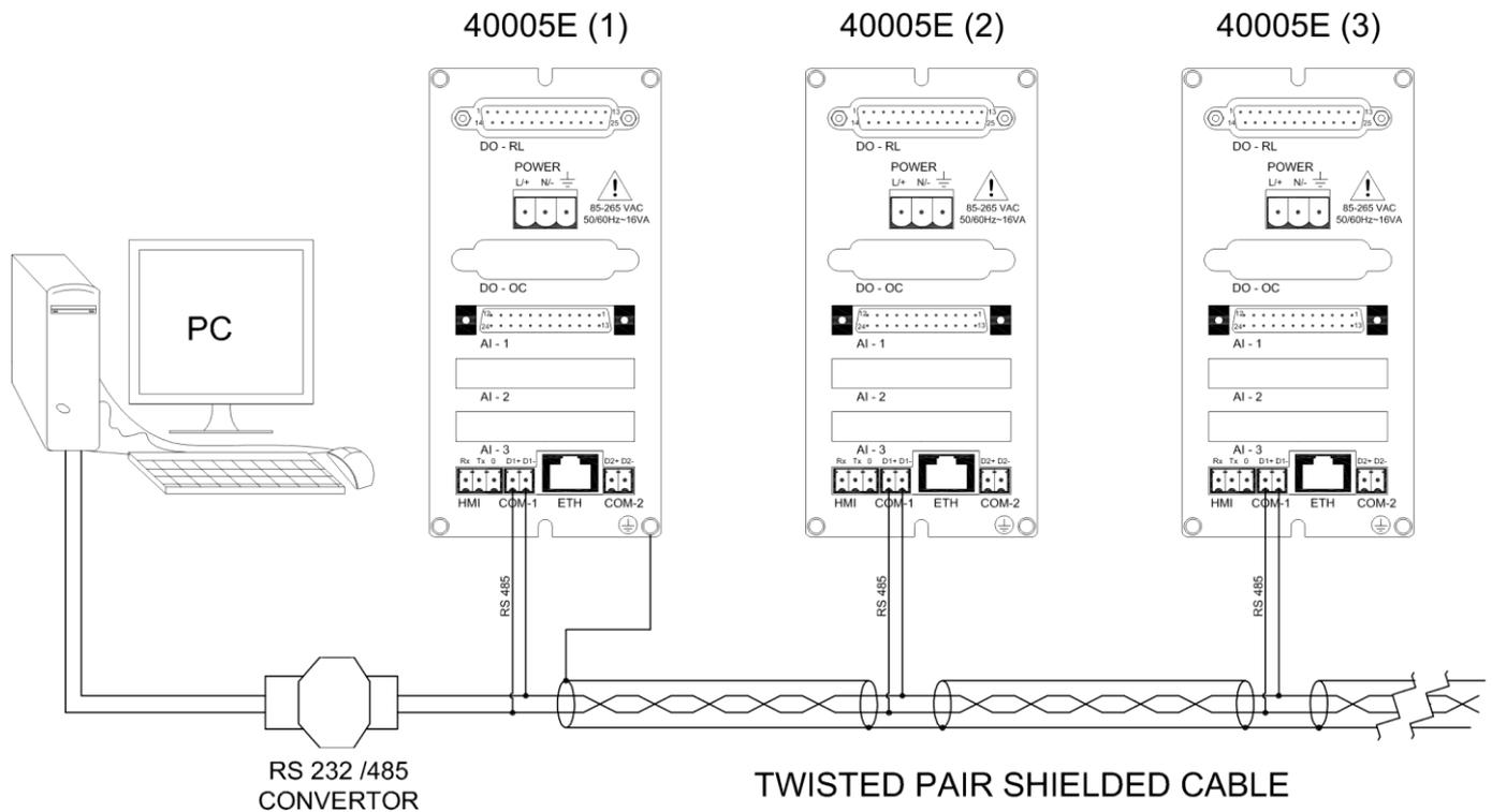
**Figure 10 Communication Cable Connections**
