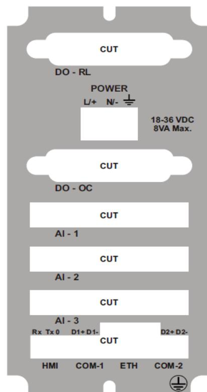
Figure 5 Rear Panel Diagram for DC Supply
