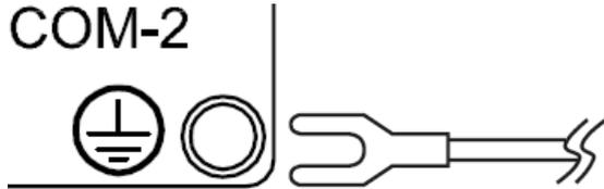
Connect the protective conductor terminal to earth, Use a spade lug to make contact with the metal surface of the 40005E.
