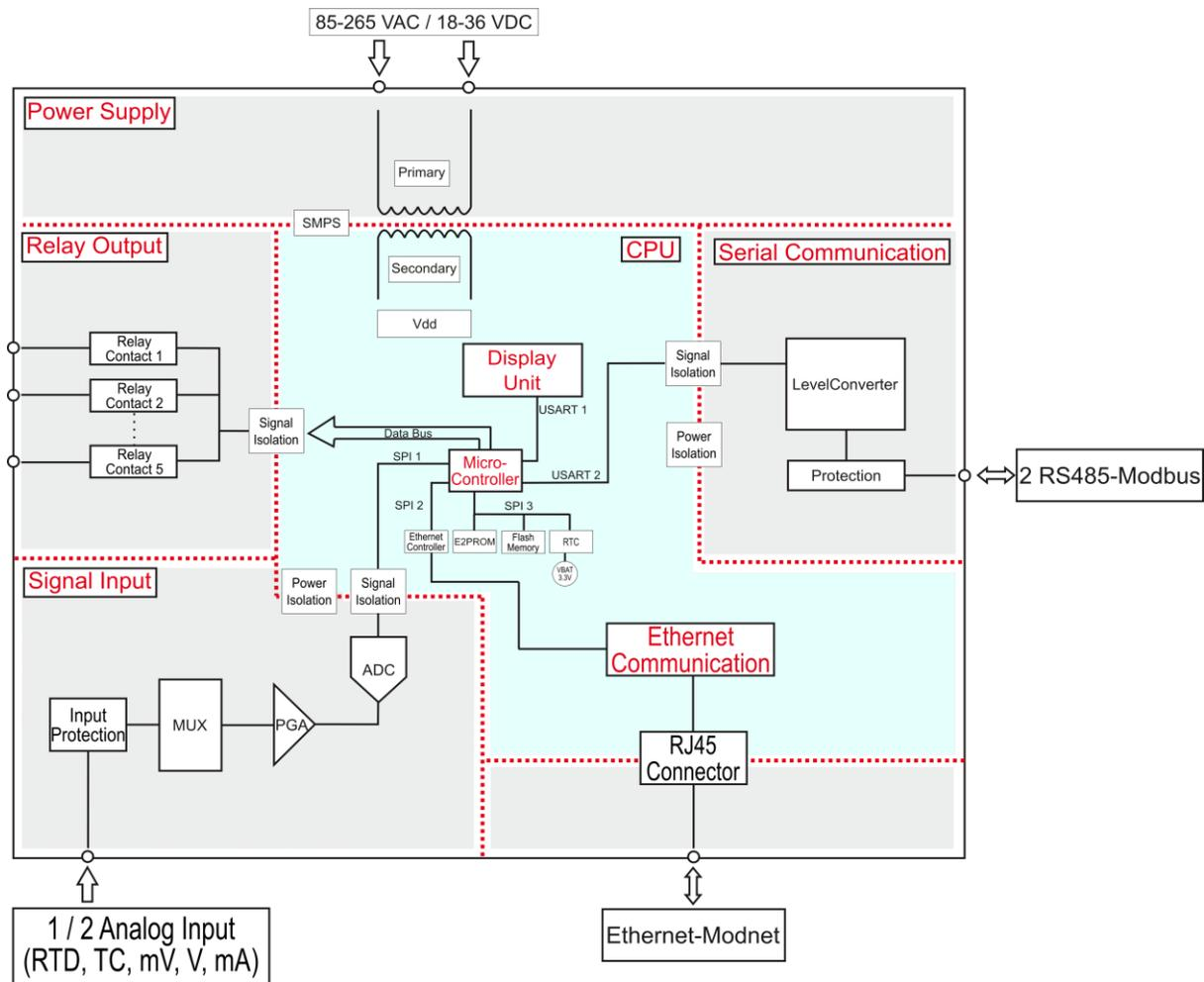
**Figure 11 Functional Block Diagram of 40005E**
