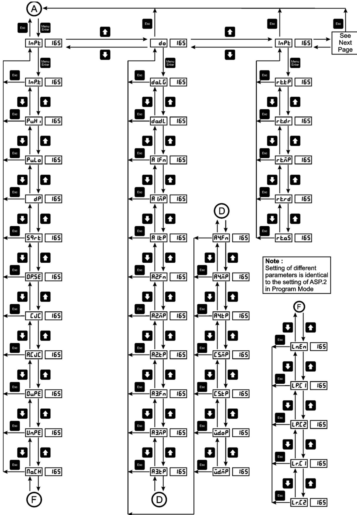
Figure 13 Configuration Mode Flow diagram
