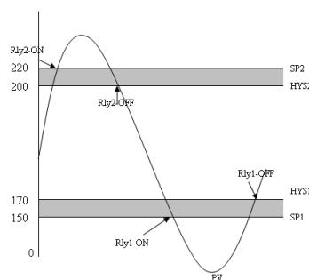
Relay 2-ON till PV>SP2+HYS2 after that Relay 2- OFF.
