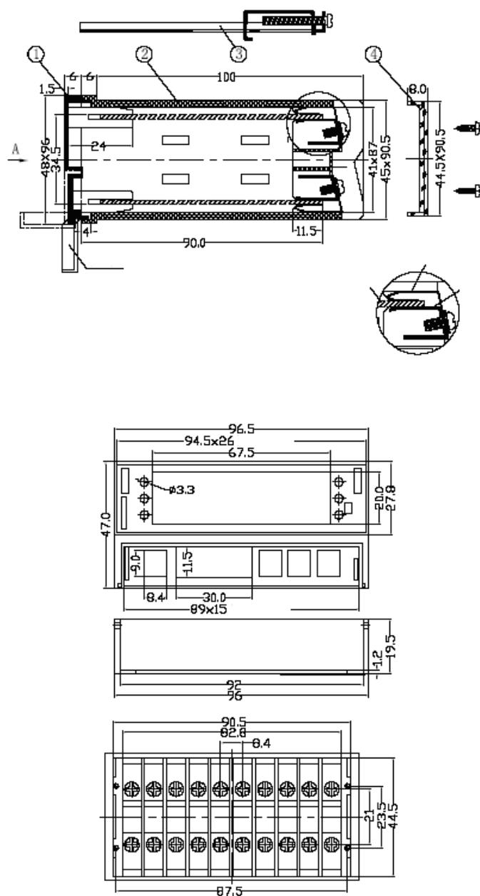
Fig 4.1.Panel cut out for 409-W
