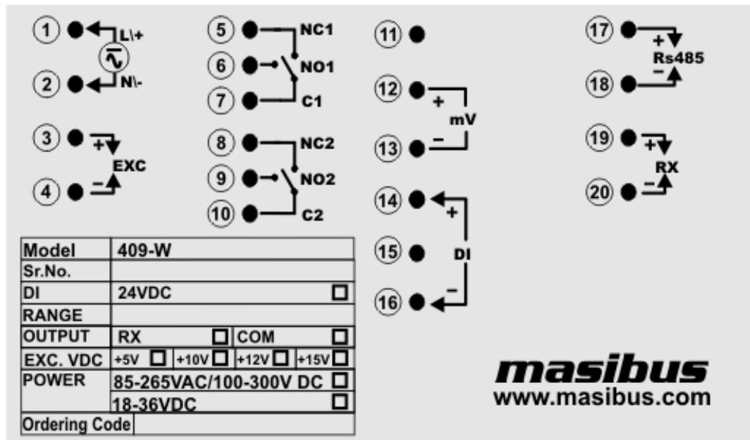
Fig 5.1. Terminal arrangement for 409-W
