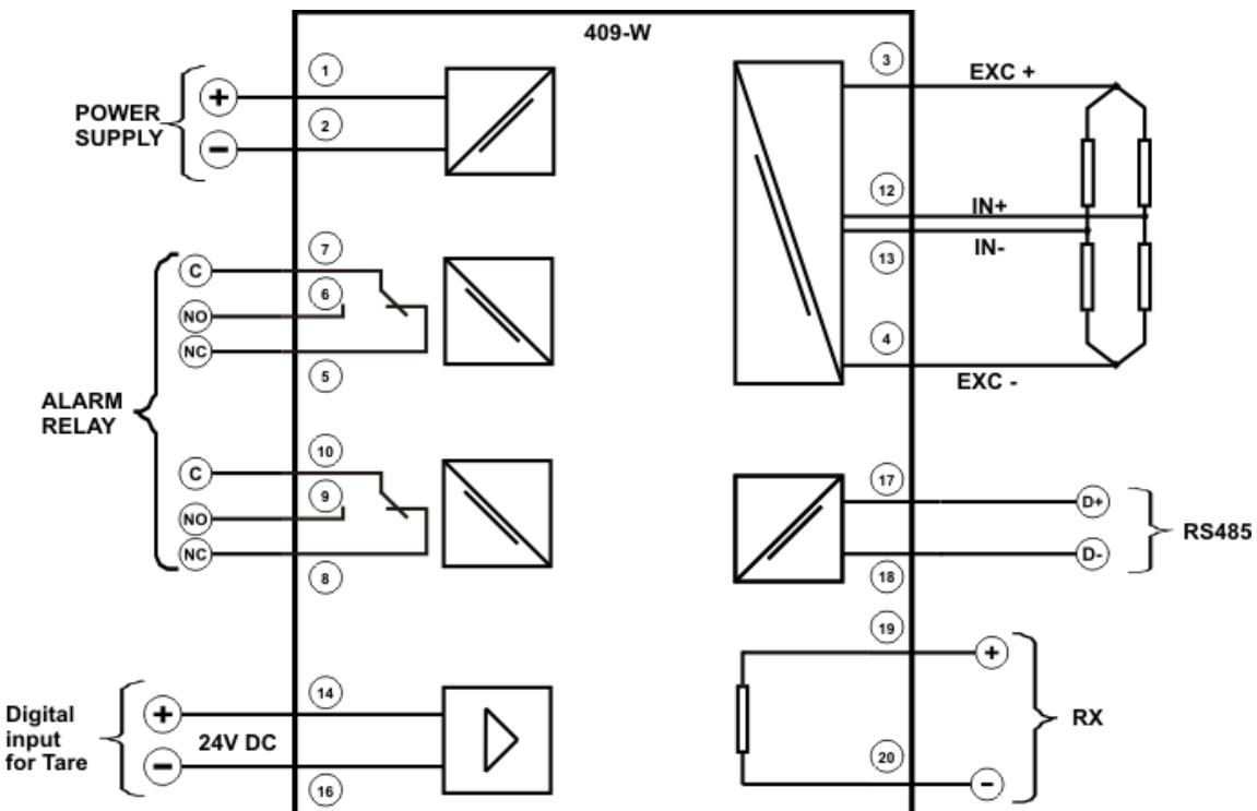
Fig 5.2. Connection diagram for 409-W
