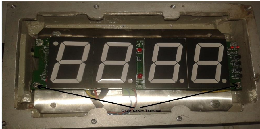
Figure 21 Open Screw Terminal of DDU-24-XP
