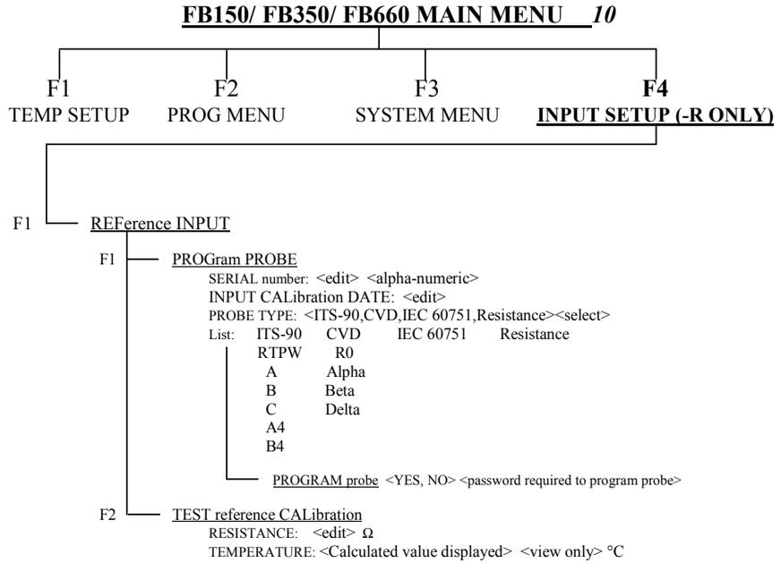
**Figure 13** Main Menu - Input Setup
