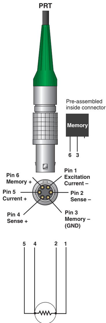
**Figure 8** Probe connector wiring
