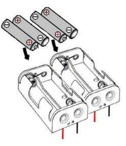
**Step-4**Make sure battery polarity match with respective battery holder before insertingnew battery. Switch on unit after inserting new battery. Make sure device onproperly by looking display parameters.follow reverse procedure do boxing and mounting of unit on back-plate.
