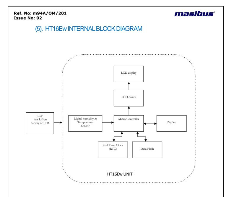
Fig 1: Block Diagram of HT16Ew
