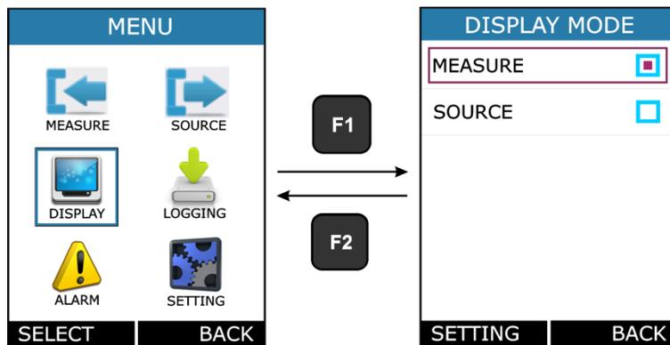
There is mainly Two RUN Display Mode possible in this device. And this mode can be selected from the above Page. What information to be shown in each RUN Display Mode can be defined by this page.
