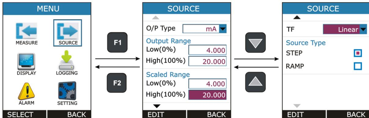
This page contains parameters related to Measure like Output Type, Output Range, Scaling, Transfer Function Step and Ramp. The Description of the Parameters appear on this page is given below.
