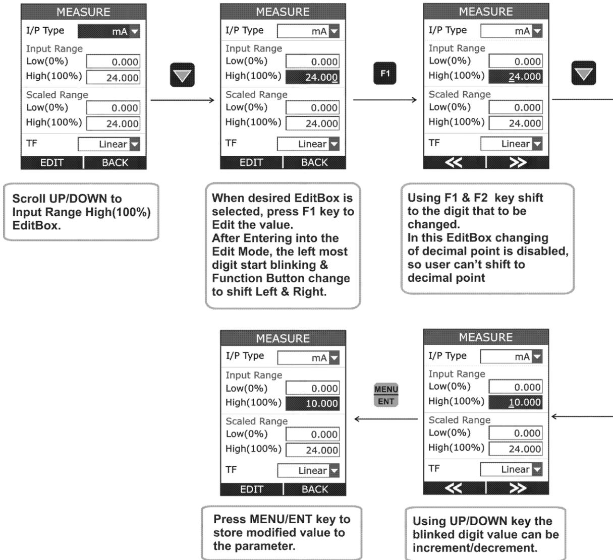
The above figure shows the example how to change Input High(100%)Range from 20.000 to 10.000 mA.
