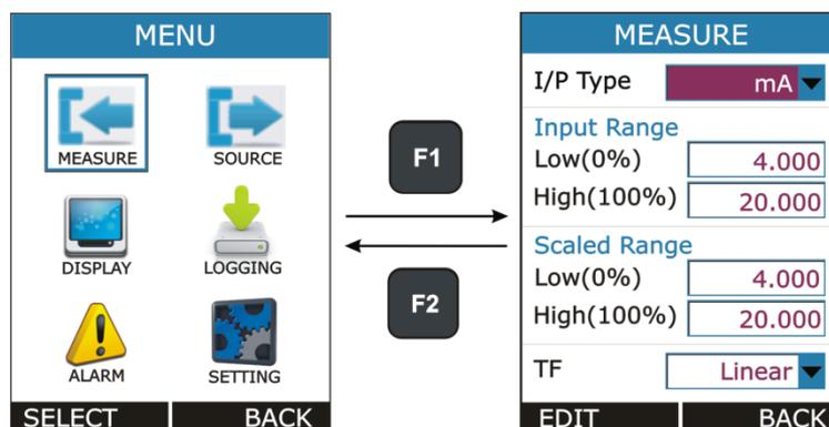
This page contains parameters related to Measure like Input Type, Input Range, Scaling and Transfer Function. The Description of the Parameters appear on this page is given below.
