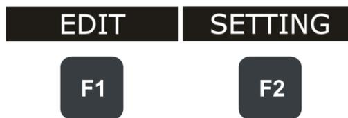
The Function Key Bar at the bottom of the display is visible all the time. There are 2 Function Key Available. The meaning of the Function Keys varies depending on the situation. A Blank Function key text means that the function is disabled at the moment.
