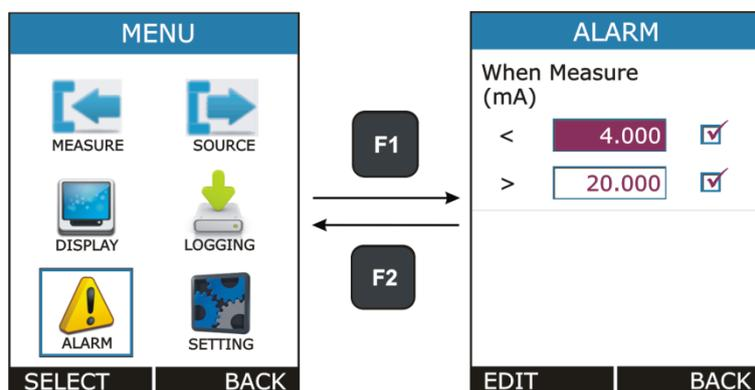
Individual alarm limit values may also be enabled/disabled using the check box preceding the alarm limit value.
