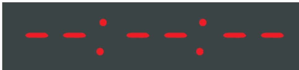
Figure 19 Startup Operation when Unit is Power On
