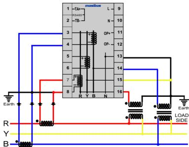
2B) 3-Wire 2- Element Direct Connection Using 2CTs
