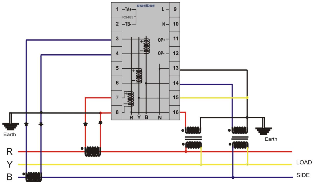
**b) 3-Wire 2- Element Direct Connection Using 2CTs**
