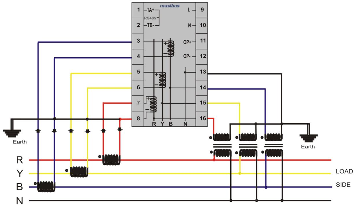
**b) 4-Wire Wye-3 Element Direct Connection Using 3CTs**
