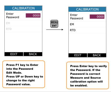
To calibrate the instrument first enter the correct password. If the entered password is correct Measure & Source Calibration option will be enabled.
