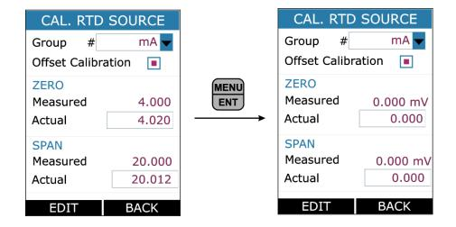
• To enter into the Offset Calibration, Select the **Offset Calibration** radiobuttonboxinCAL. RTD SOURCE page.
