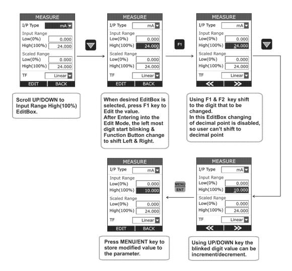
The above figure shows the example how to change Input High (100%) Range from 24.000 to 10.000 mA.
