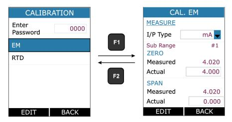
For Better Calibration Input Range is divided into two sub ranges. So For each input type, Calibration of both sub ranges need to done. The Sub Ranges of each input type is given in the below table.
