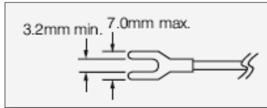
**Fig 4.3: Lead Termination Detail**
