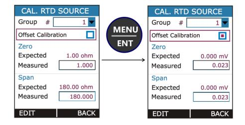
• To enter into the Offset Calibration, Select the **Offset Calibration** Radiobuttonbox in **CAL. RTD SOURCE** page.
