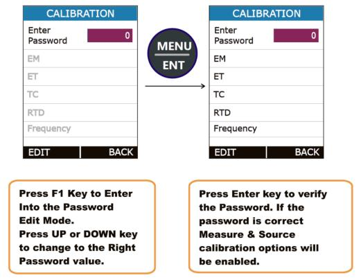
To calibrate the instrument first enter the correct password. If the entered password is correct all other options will be enabled.
