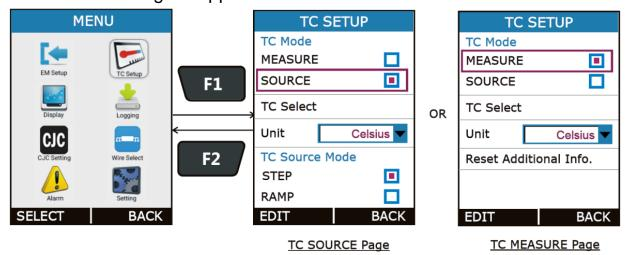
This page contains parameters related to Thermocouple like TC Mode Type, TC Type, Unit, TC Source Mode etc. The Description of the Parameters appear on this page is given below.
