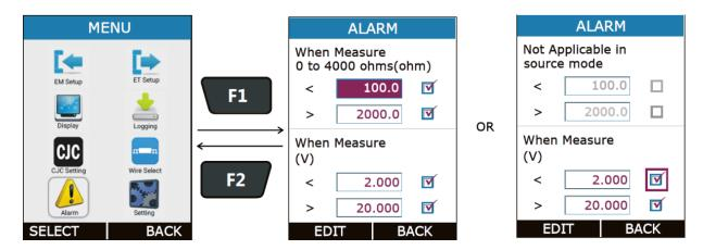
Individual alarm limit values may also be enabled/disabled using the check box preceding the alarm limit value.
