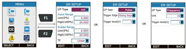
This page contains parameters related to EM Measure like Input Type, Input Range, Scaling and Transfer Function. The Description of the Parameters appear on this page is given below.
