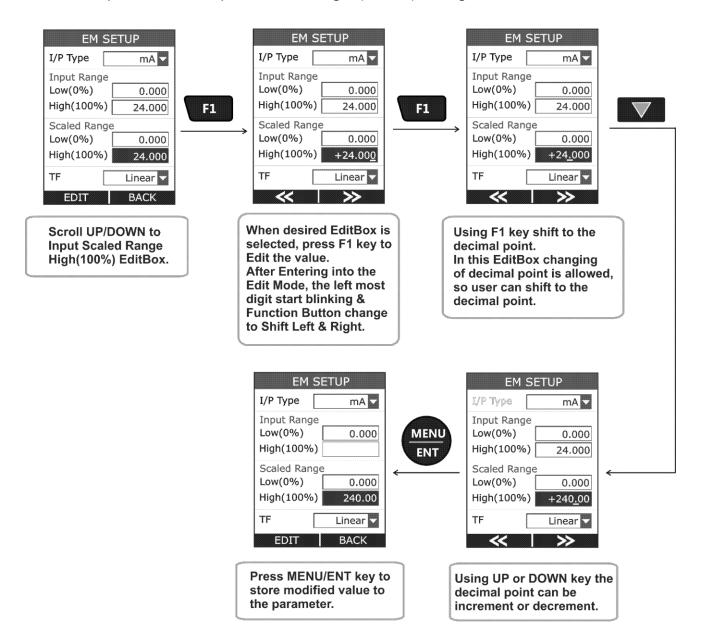
To change the sign of the value, shift to the sign digit and pressing UP or DOWN key will toggle the sign.
