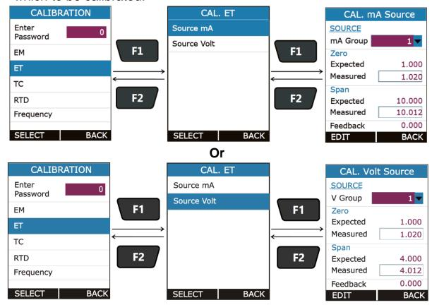
• Expected Values of Zero and Span for source calibration are as per below table.
