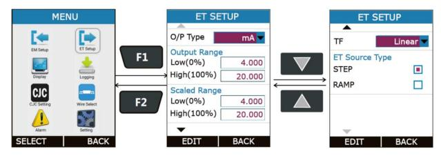
This page contains parameters related to ET like Output Type, Output Range, Scaling, Transfer Function Step and Ramp. The Description of the Parameters appear on this page is given below.
