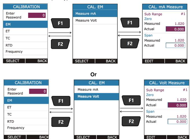
For Better Calibration Input Range is divided into two sub ranges. So For each input type, Calibration of both sub ranges need to done. The Sub Ranges of each input type is given in the below table.
