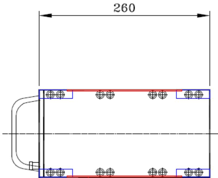
Figure 5 : VMS-R chassis side view dimensions
