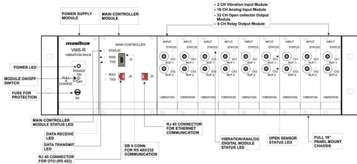
Figure 2 : System setup for VMS-R with Ethernet communication (Full 19")
