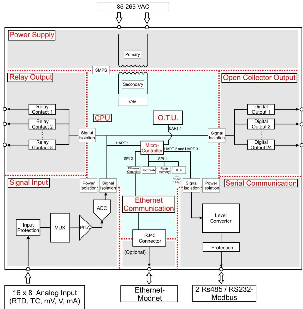
Figure 13 : VMS-R system block diagram
