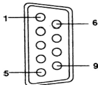
Figure 12 : Port J1 and J3 RS 232 communication wiring and cable detail
