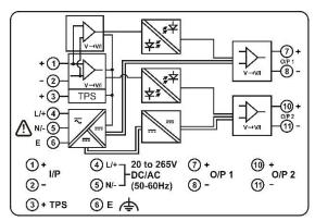
Block Diagram Connection Details SOP HART Pass Suitable for 2 wire transmitter only (Aux Powered)  $% \left( A_{1}^{2}\right) =0$
