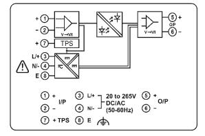
Block Diagram and Connection Details of DOP (Aux Powered)
