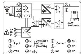
Block Diagram and connection details of DOP HART Pass Suitable for 2 wire transmitter only (Aux Powered).
