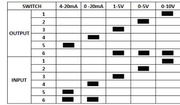
Switch Selection Table for Different type of Input/Output
