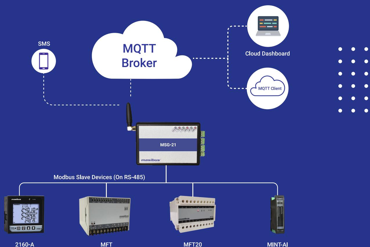
REMOTE MONITORING OF ELECTRICAL SYSTEMS - IIOT APPLICATION
