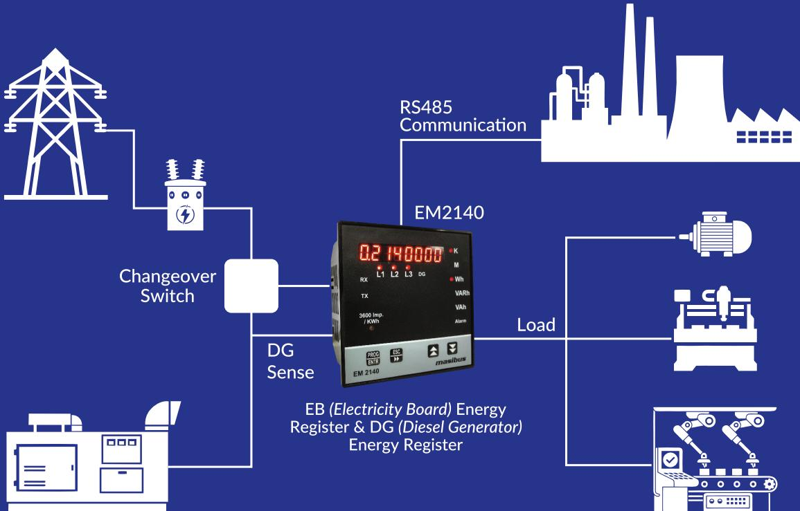
MONITORING FOR EB/DG USE & MEASUREMENT
