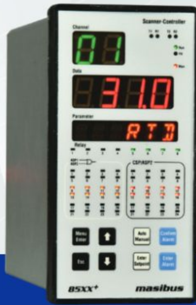
85XX+ (8/16/24-Channel Scanner & Data Logger)
