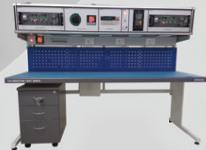
Electrical Test Bench
