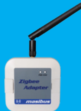
MSC-ZB-RS (RS-485 Serial to ZigBee Wireless Converters)
