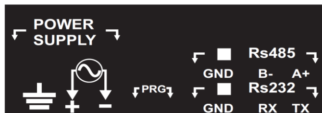
Figure 19 Connection on Terminal plate of DDU-TM-44/46 or DDU-44/46 Wall Mount
