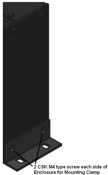
Fig 4.4.5: CSK screw fitting information for Table Top Clamp
