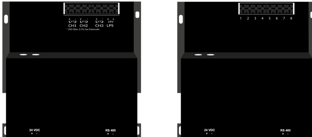
Fig 4.1: Terminal Connection Detail of CDU
